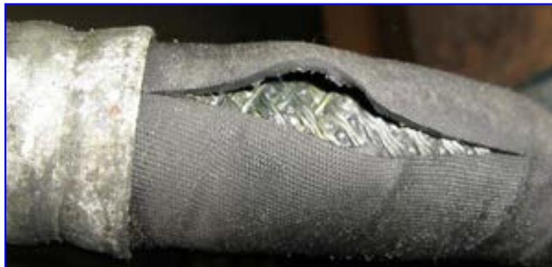
This is an air conditioning line that has the outer covering ruptured. This line may be holding pressure now, but will most definitely fail. By catching this and repairing it before it fails completely, further damage to the system can be avoided.
