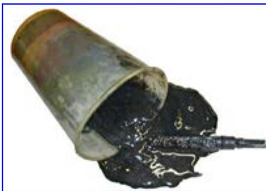
This picture is of sludge that came out of a system that had experienced catastrophic failure. Air conditioning systems should always be service by properly trained personnel. Most para-transit vehicles have a rear system, installed by the body manufacturer, which is integrated with the factory system. Be sure that the person servicing the system is aware of this and knows the proper capacities.
