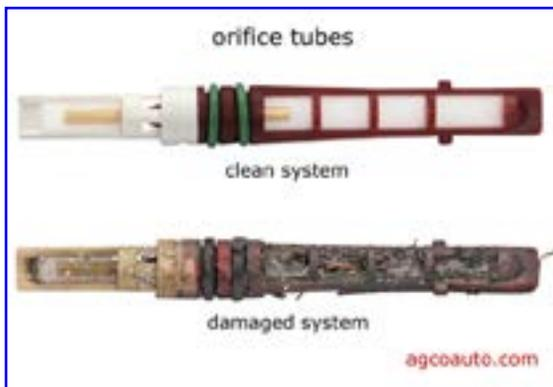
This picture shows a two orifice tubes. The orifice tube acts as a filter in the system to catch small amounts of debris. A plugged orifice will result in a high pressure reading on the gauges and a loss of cooling. A problem in the system could be detected in this manner and repaired before a catastrophic failure occurs.
