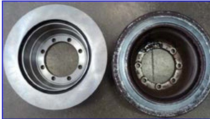
Here is an example of a new rotor compared to an old one. The flat smooth surface of the new rotor provides much greater stopping power.
